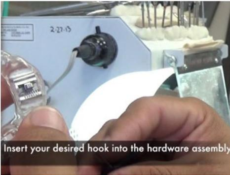
Insert your desired hook into the hardware assembly
