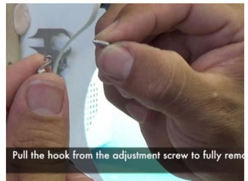
There is a small clear/white washer on the end of the screw. Remove and store. We will need it when putting back together. Next, put the hood and screw back into the assembly. It will hold the hook. Now turn the screw until it fully backs out of the hook. Now you can pull the screw and hook out. It's fully disassembled.
