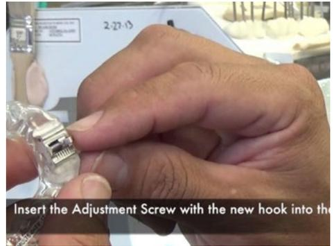
Insert the Adjustment Screw with the new hook into the
